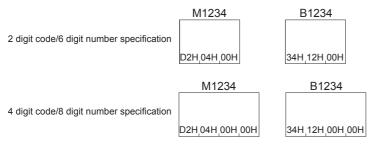
Internal relay M1234 becomes 0004D2H and is sent in the order of D2H, 04H, and 00H.
