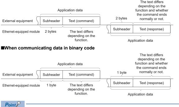
It is not necessary to set the response to a command from the external equipment by the user because the response is created and sent by the Ethernet-equipped module.
