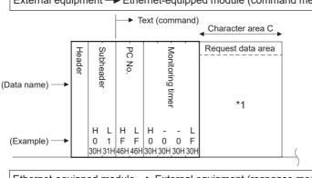
External equipment -> Ethernet-equipped module (command message)
